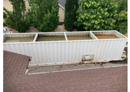
Well sand production during re-development
