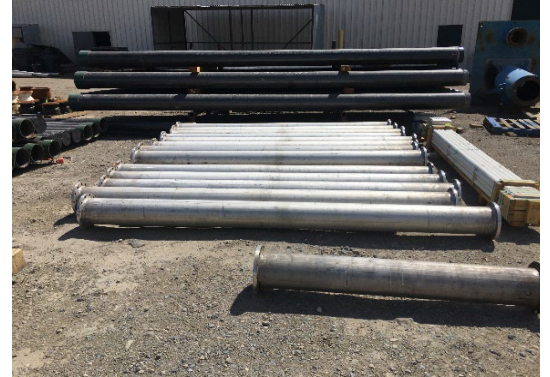
Remanufactured stainless steel column piping at fabricator
