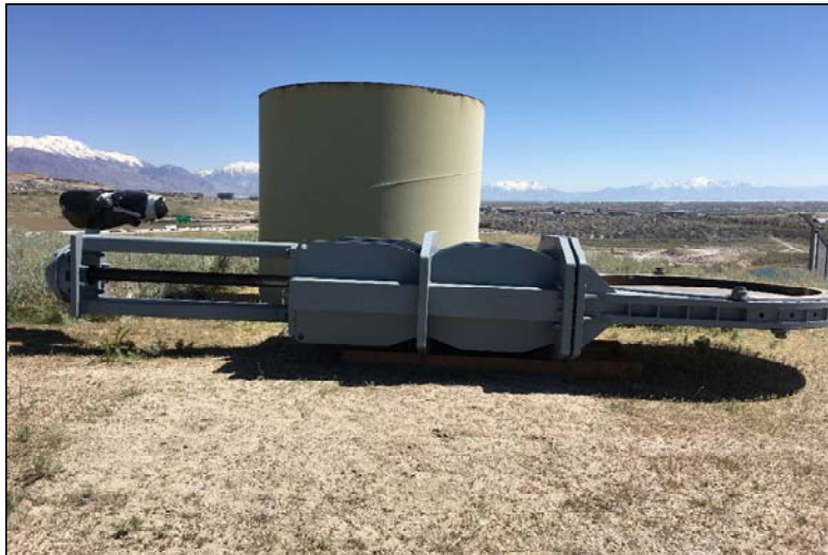
The re-built valve delivered to the flow control structure
