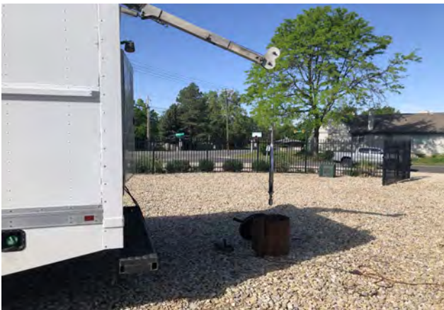
Setting up downhole video camera
