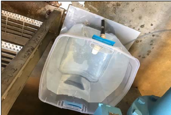
JVWCD finished water testing chamber for visual inspection of filter efficiency
