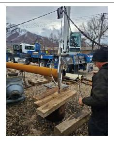
Setting up instrumentation to perform casing log
