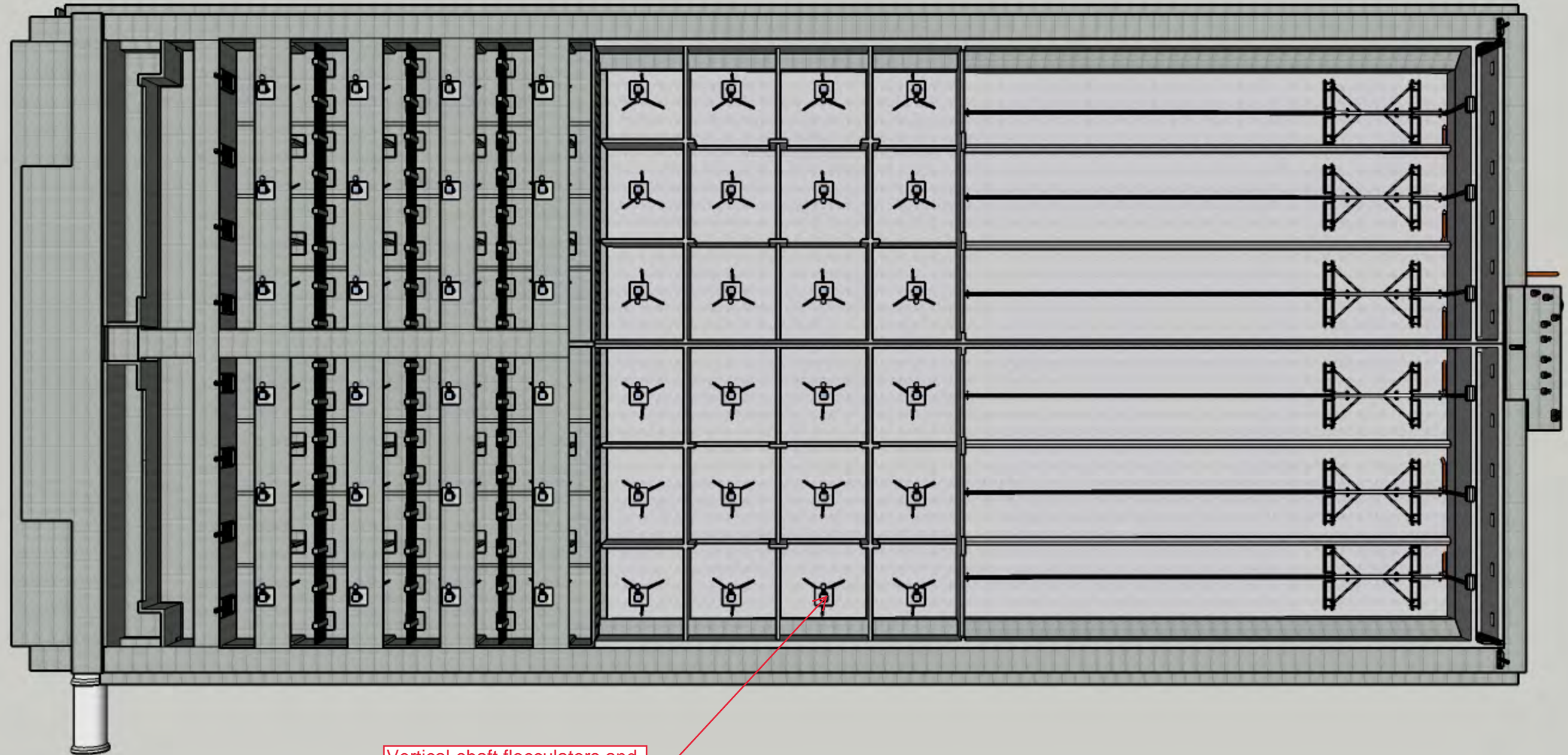
Vertical-shaft flocculators and hoseless solids collectors
