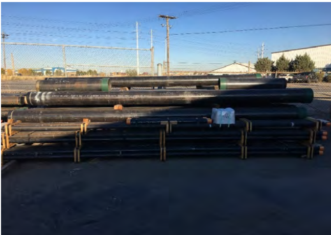
New pump shaft and column
