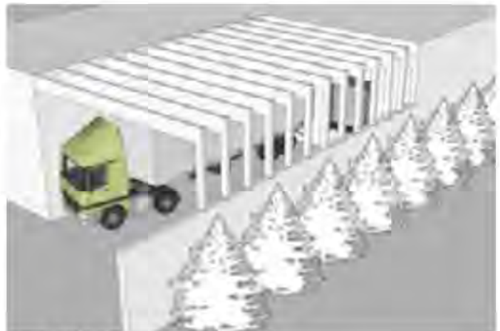
Figure 5.2 (6). Screened loading area.
