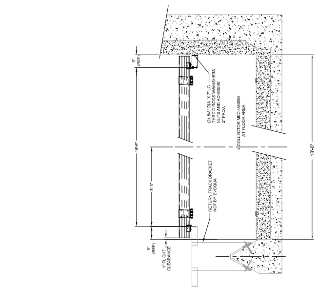
▲ TRACK CROSS SECTION VIEW OUTER TANKS 4-SHAFT FOREBAY @ KNEE WALLS & OUTER WALLS (SCALE: 1/16" = 1'-0")
