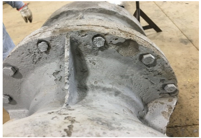
Pitting observed on old pump
