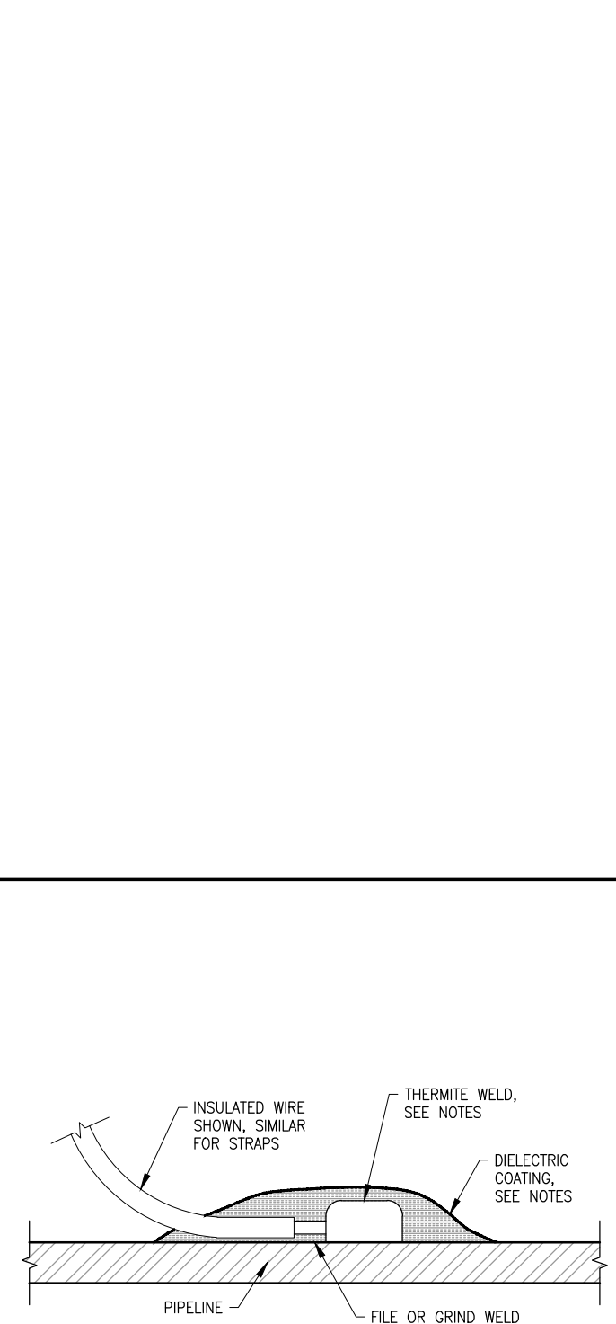
COUPLING JOINT BOND (CP 2759) NTS
