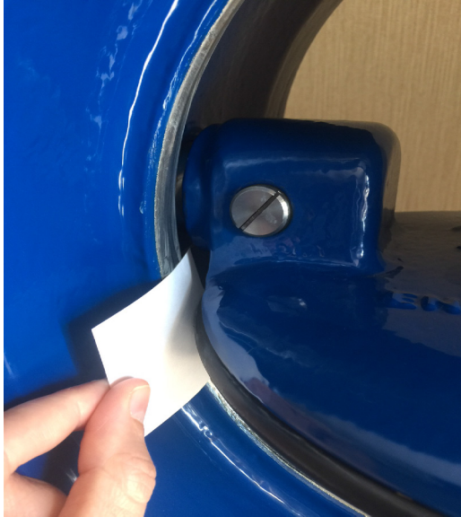
A business card is placed between the NiCr welded body seat and resilient seal showing a true double offset design.
