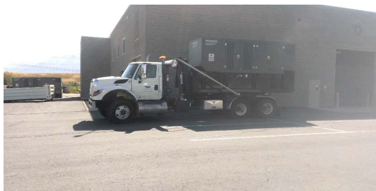
Generator unit staged on "hook-lift" truck for transportation to District facilities
